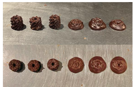
Figure 7 Chocolate samples printed with the same model (the temperatures from left to right were 29°C, 30°C, 31°C, 32°C, 33°C, and 34°C)
