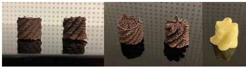
Figure 5 The front and perspective views of two dark chocolate samples (the left with a frequency of 9 and amplitude 0.1, and the right with a frequency of 7 and amplitude 0.4), and the perspective view of a white chocolate sample (it deformed at the base due to its softer texture)
