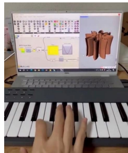
Figure 4 The model shape in Grasshopper changes according to the pitch of the MIDI notes played
